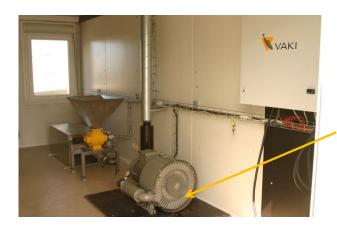
The feed is picked from the airlock by air from the blower and transports it through the feeding pipes to the cages.
