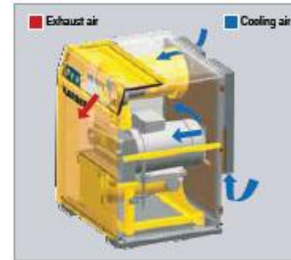
AIR FLOW COOLED WITH AIR COOLER
